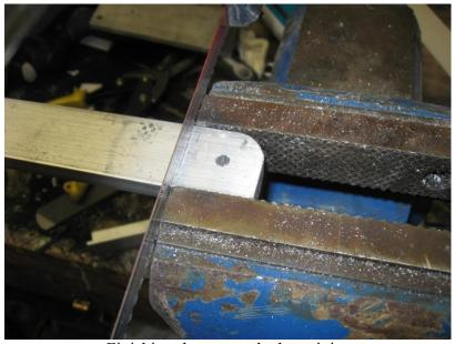
Finishing the cut on the knee joint
