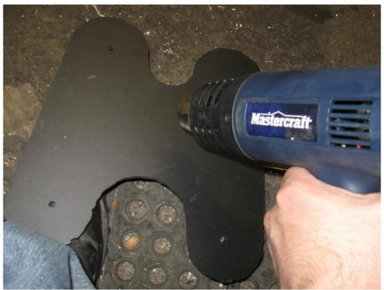
Heating the Center of the Lower leg Sintra Shape
